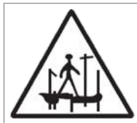
Danger Scaffolding Incomplete
